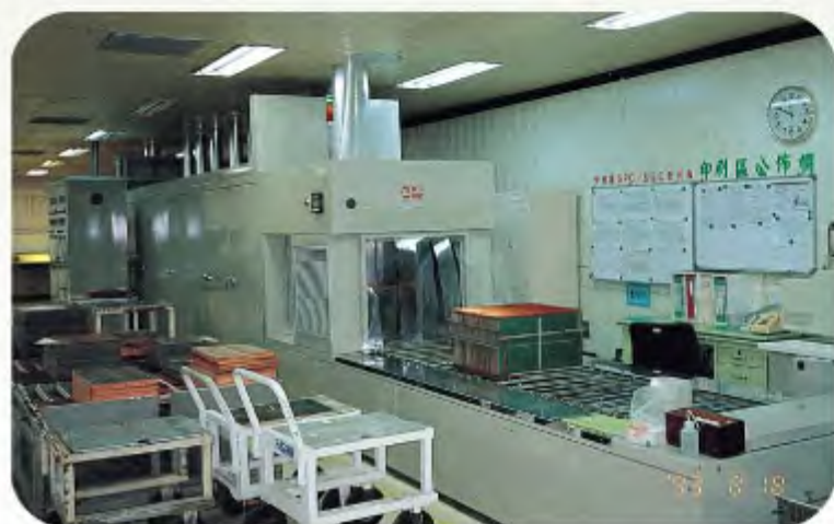
框架式自動熱風輸送爐 Automatic Hot Air Conveyor Oven (Rack Type)
