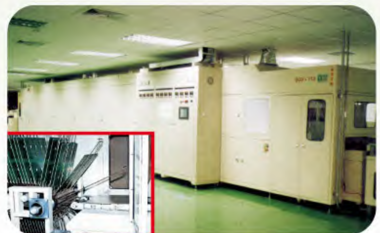
板架式自動熱風輸送爐 Automatic Hot Air Conveyor Oven (Wicket Type)
