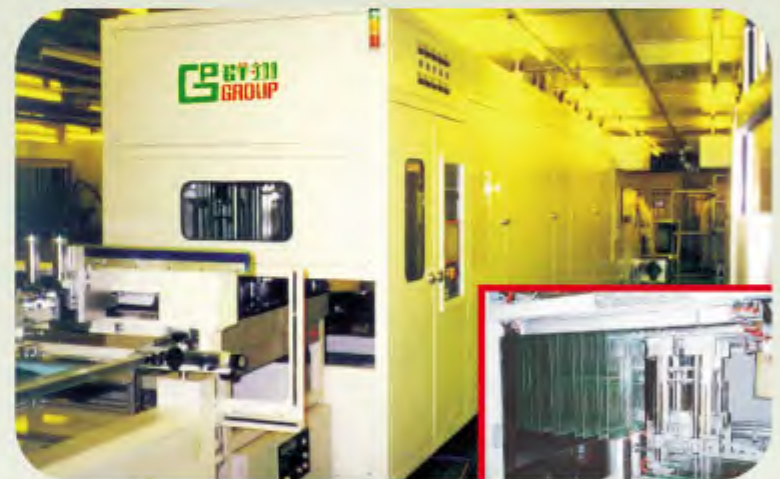
懸吊式自動熱風輸送爐 Automatic Hot Air Conveyor Oven (Gripping Type)
